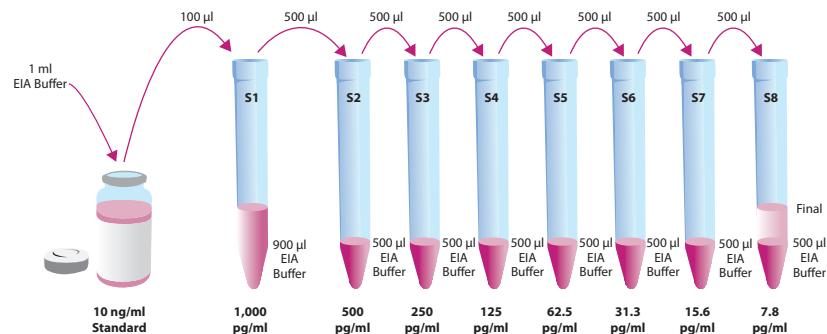
Figure 6. Preparation of the PGE<sub>2</sub> standards
