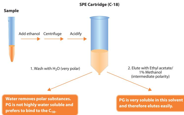
Figure 5. Schematic of PGE<sub>2</sub> Purification by SPE (C-18)
